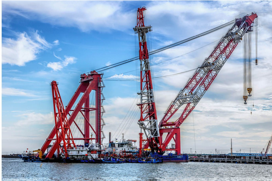
浮吊 Floating Crane
